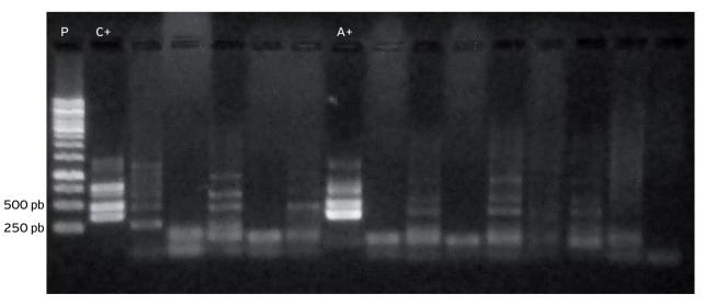
P: Standard, molecular weight 1 Kb; C+: positive control, obtained after DNA extraction from a cellular cultivation of *A. phagocytophilum*; A+: positive sample; two last gutters as filled with the white reaction from first and second reactions, respectively.
