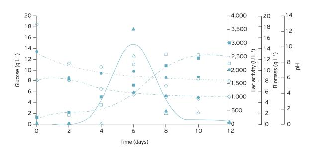
**Figure 2.** Profiles of biomass growth (dashed line,  $-\blacksquare$ -,  $-\Box$ -), glucose consumption (dotted line,  $-\bullet$ -,  $-\bigcirc$ -), laccase activity (continuous line, -▲-,  $-\triangle$ -) and pH (dash dot line,  $-\bullet$ -,  $-\diamondsuit$ -) with time (days), in the presence of 7.5% Tween 80. The open and closed symbols represent data from duplicates.
