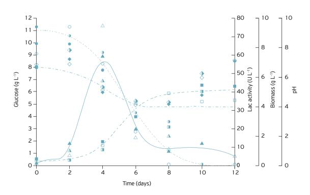
**Figure 1.** Profiles of biomass growth (dashed line,  $-\blacksquare$ -,  $-\Box$ -), glucose consumption (dotted line,  $-\bullet$ -,  $-\bigcirc$ -), laccase activity (continuous line,  $-\blacktriangle$ -,  $-\bigtriangleup$ -) and pH (dash dot line,  $-\blacklozenge$ -,  $-\diamondsuit$ -) with time (days), in the absence of Tween 80. The open and closed symbols represent data from duplicates.
